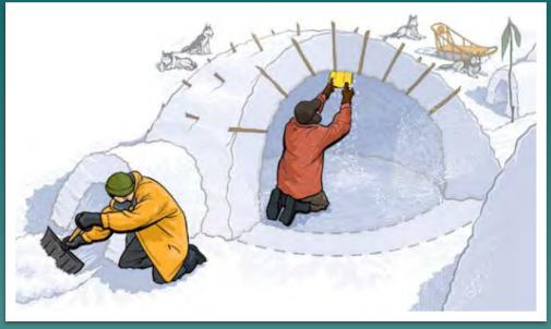
Channel in floor draws cold air out the door
